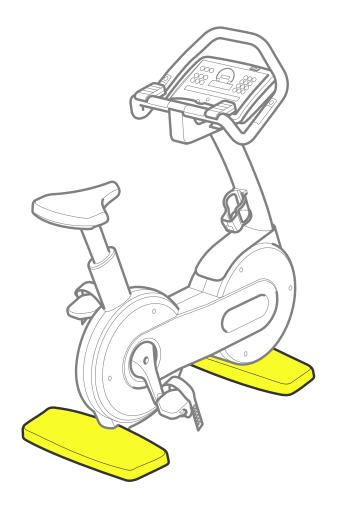
**Bases**: support the equipment frame and components.
